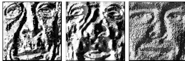
Fig. 9. Example of LATP Lower and Upper image fusion for SWIR using DWT, MWIR using SIDWT and NIR using FSD.
